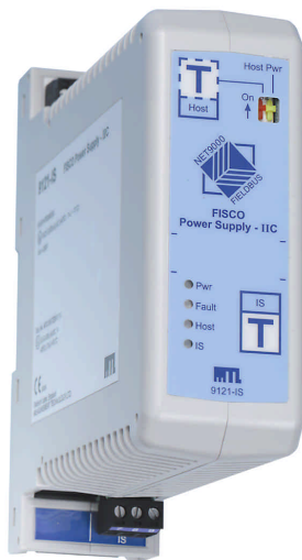
Figure 2 - FISCO power supply
